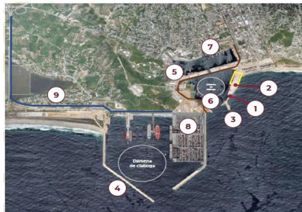
Figure 2. Development and extension work in the Port of Salina Cruz. Note: Completed work: 1 (multiple use pier construction). In progress: 2 (reinforcement of pier and container terminal), 3 (enlarge the access and sheet piling of pier) and 4 (break water construction). Not started: 5, 9 (rail and road access to container terminal), 6 (dredging of navigation area), 7 (traffic control center and rearrangement of land access), 8 (specialized container terminal).
