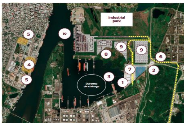
Figure 1. Development and extension work in the Port of Coatzacoalcos. Note: Completed work: 1 (new dock), 2 (road access) and 3 (construction dredging). In progress: 6 (rail access), 7 (urbanisation service) and 8 (Ethane terminal). Not started: 9 (LNG terminal) and 10 (Specialized container terminal).
